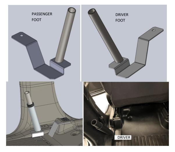
7.) Insert partition (part number begins with TP-E, differs depending on configuration) into vehicle through rear doors and set on floor. Lift partition, tilt top of partition toward rear of vehicle, and slide partition tube onto mounting feet. Insert two 3/8-16x1 screws into B-pillar brackets as shown to hold partition in place. Tabs on partition tube sit outboard of pillar brackets. Lower partition tabs are not used.
