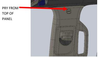
3.) Separate driver and passenger upper and lower B-pillar trim panels by prying lower trim outward at seam. Mounting pin locations are marked below. Side shown is driver side. Fully detach the upper trim from the B-pillar and set it aside.
