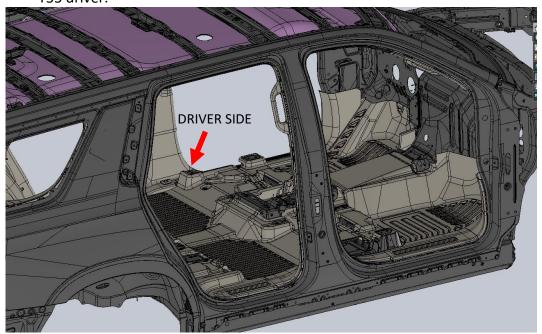
2.) Remove driver and passenger "airbag" plastic cap from upper B-pillar trim using body panel removal tool or flat blade screwdriver. Remove screws behind panel using 7mm socket.
