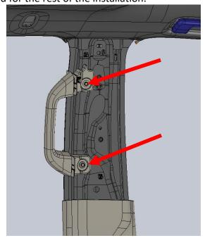
5.) Mount B-pillar brackets (#dbpb, #pbpb) to B-pillars where handles were mounted using original M6 mounting hardware removed in step 4. Replace trim and re-insert screws removed in step 2 using 7mm socket. Bracket is shown installed on driver side.
