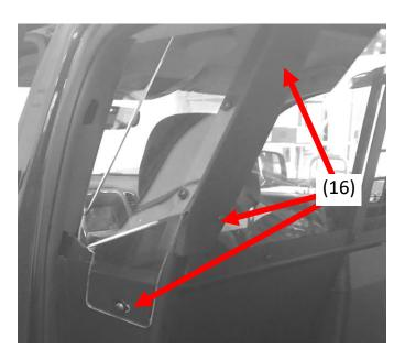
17.) Repeat steps 14-16 on the opposite side of vehicle, securely tighten all seat bolts to O.E.M. specification and securely tighten all partition fasteners.
