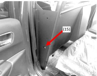
15.) Temporarily support partition, remove  $3/8-16 \times 1-1/2$ " bolt and install lower metal wing. Loosely attach lower wing to lower partition tab using the provided  $3/8-16 \times 1$ " bolt, washer and nut.
