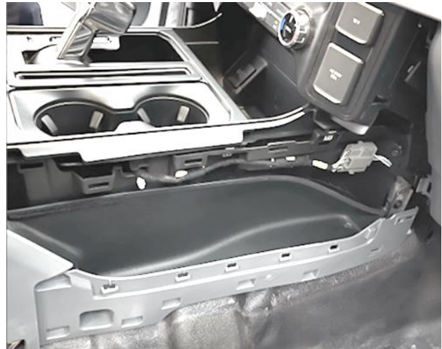
Lower and upper trim panels removed
