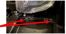
2.) Remove the plastic cover from the B-pillar handle and remove M6 fasteners using an 8mm socket. Install B-pillar handle bracket (#bp) using bracket spacers (#spc) and two M6-1x40 button head socket caps with ¼ washers, provided.
