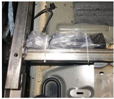
6.) If a wiring harness channel is present in the second row footwell, remove it with a 4mm allen wrench. There are four M6 fasteners holding it in place. Save the fasteners.
