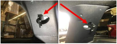
6.) Install the lower panel (large flange down and facing toward the rear) in the vehicle and attach to the (2) front bracket study using the (2) provided ¼-20 nuts. Tighten nuts securely.
